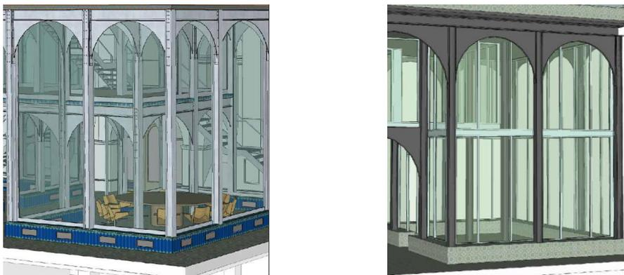
Figure 2 a) Architectural intension (left), b) standard fire resistant glazing system with intermediate transom (right).
