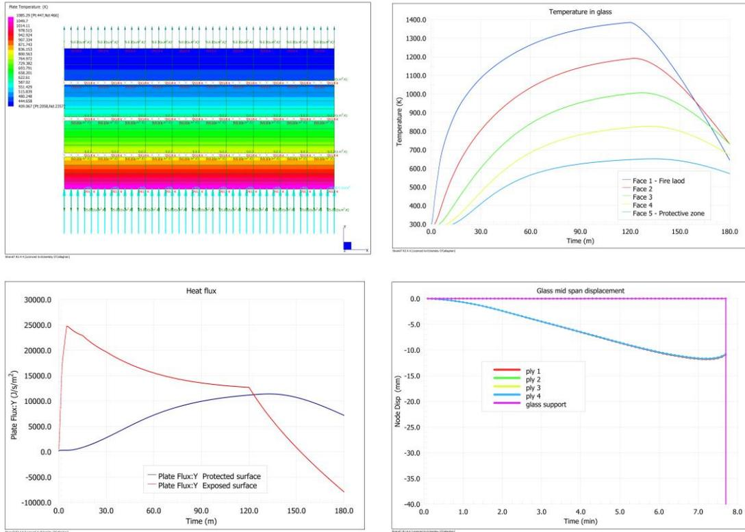
Figure 3 a, temperature plot at 30 min, b. temperature vs. time, c. heat flux vs. time, d. deflection vs. time
