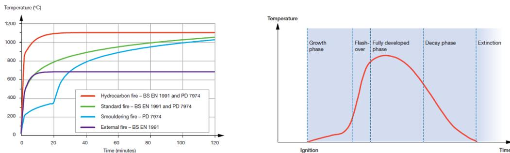
Figure 1a.) Standard fire curves, b.) Real fire stages
