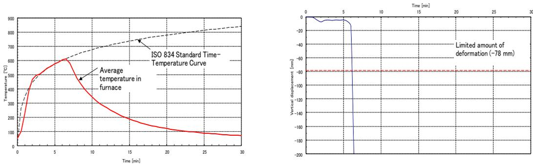
Figure 4 a) Measurement of temperature in furnace, b) Time-vertically displacement relationship
