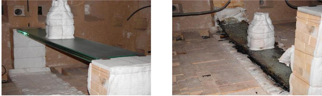
Figure 5 a) Glass component before and b) after fire resistance test
